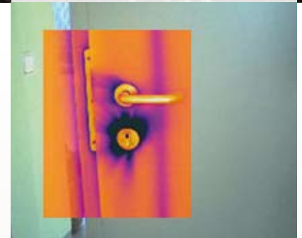
Air leaks in door with considerable temperature difference
