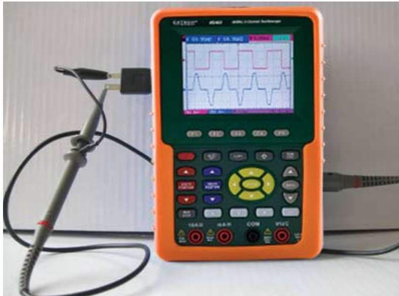
Fig 39: Square-wave test signal
