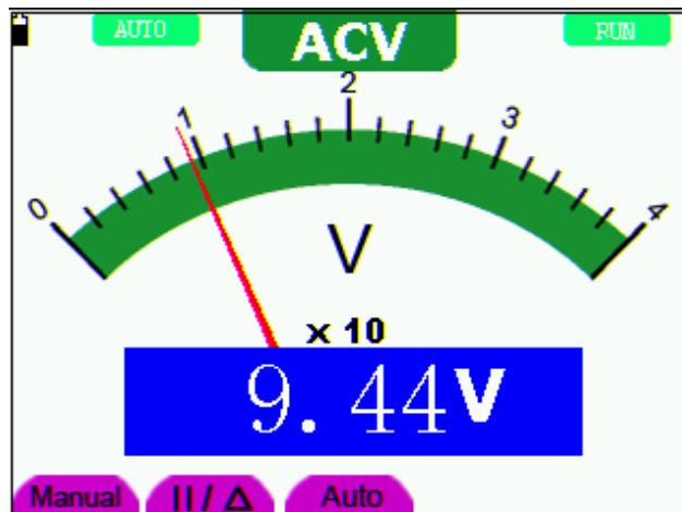
Figure 7: AC Voltage Measurement
